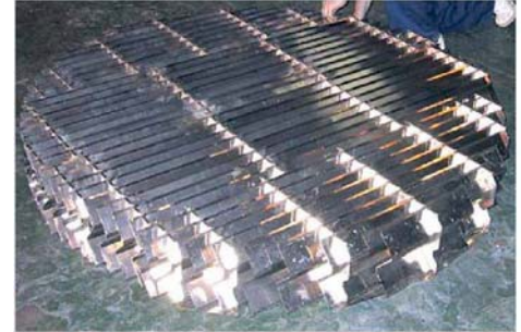
Vane Demister Type 3-2-NH 1600--2400mm Ø IPA Absorber Column MOC Nickel200
