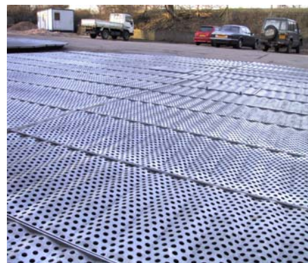
Ripple Trays 5791mm Diameter Ethylene Quench Tower / Primary Fractionator
