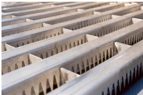
Disc and Donut Trays - Bundle Construction 2600mm Diameter Deaerator Tower
