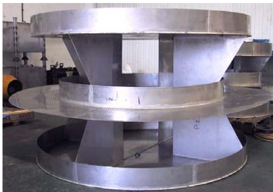
Disc and Donut Trays - Bundle Construction 2600mm Diameter Deaerator Tower
