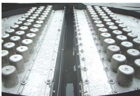
Bubble Cap Trays, Slotted Type 1829mm Ø Vacuum Flash Tower
