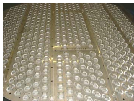
LCD Valve Trays 2273mm Ø Tifane Elimination Column
