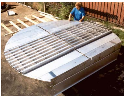
Uniflux (Tunnel Cap) Trays, 3658mm Diameter Rerun Main Column
