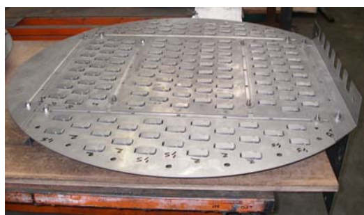
RMV60 Valve Trays 1450mm Ø MeOH Dryer Column
