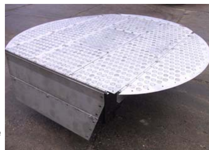
STD Valve Trays 2700mm Ø MCB Elimination Column
